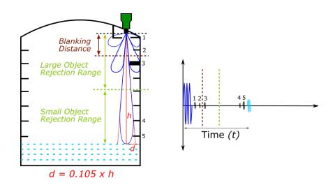
Hence, for best performance it is highly recommended to install the sensor at a distance(d) away from any unwanted objects with respect to their depth(h) satisfying the formula  $d = 0.105 \, x \, h$ , though the sensor has an *intelligent adaptive echo detection technology*' to avoid any such stray reflection echoes as much as possible with respect to the selected 'mud-pit size' or range.
