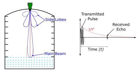
The top-mounted sensor emits a high-frequency (50kHz) ultrasonic sound pulse of very short duration, then records the time it takes for the echo to return. Based on the speed of sound for the ambient temperature evaluated by the sensor, the distance from the sensor to the top of the liquid media can be calculated by
