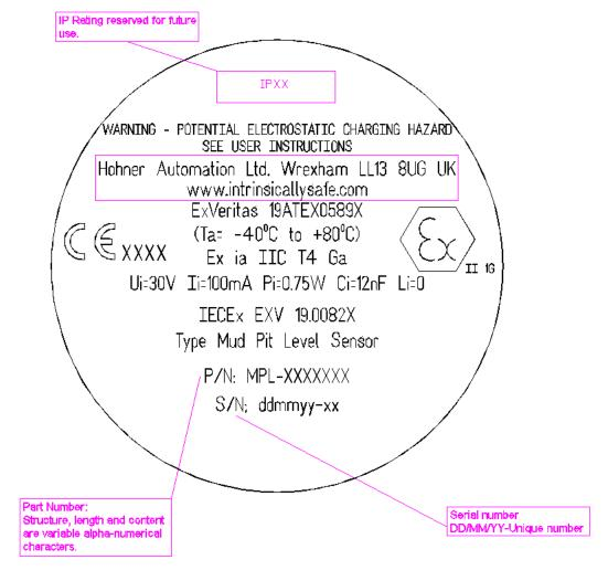
Please note that the entity parameters shown above, do not include any termination parameters (refer to termination parameter section). Part number and temperture rating are variable.
